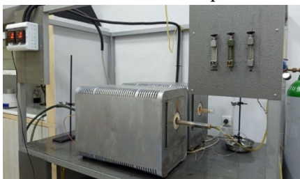
Figure 1. CVD installation for environmentally friendly synthesis of carbon nanotubes.
